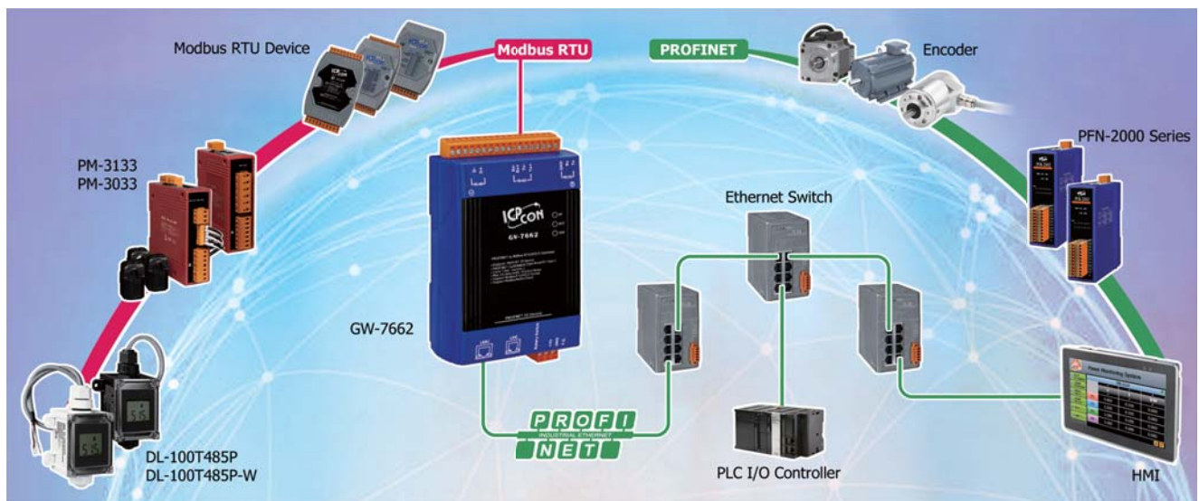
▲GW-7662 can connect PM-3033/3133/3114/3112 device and other ICP DAS's Modbus RTU slave modules in the same time.
