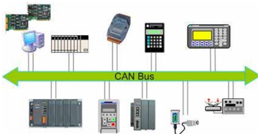
Figure 1.1 Example of the CAN network
