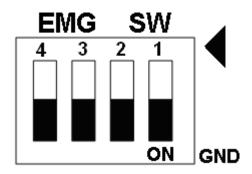
Fig. 3-13 EMG SW setting for normally GND (Default setting)
