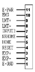
Fig. 1-7 Pin definition for CN1 ~ CN4
