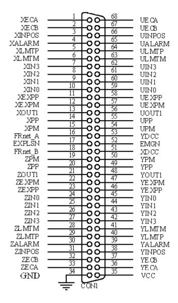
Fig. 3-2 I/O connector pin assignment for the CON1
