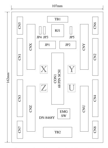
Fig. 3-1 Board layout for the DN-8468YB
