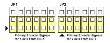
Fig. 3-11 Primary encoder signals setting
