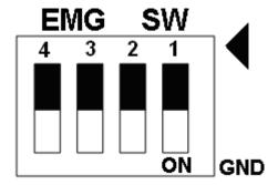
Fig. 3-14 EMG SW setting for user controlled signals.
