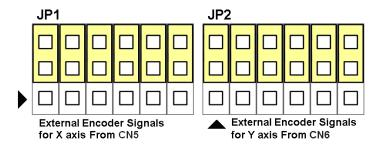
Fig. 3-12 External encoder signals setting
