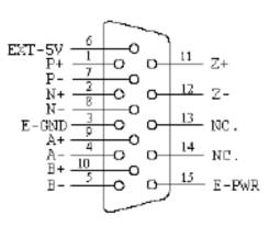
Fig. 3-8 Pin definition for CN5 ~ CN8
