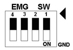
Fig. 1-9 EMG SW setting for user controlled signals.
