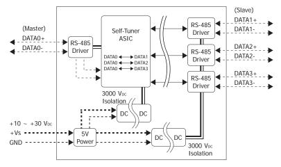
The following block diagram shows how I-7513 was designed as independent channel. Data coming from the master input will be transmitted to all four RS-485 slave channels. But data coming from the slave channels will be returned to the master input only. Thus reduces the possibility of interference between each RS-485 slave loop and makes the RS-485 networks more robust and reliable.
