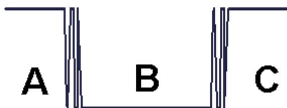
If we just use the read digital input status command to read the signal and we cannot send the command during the B period due to some reasons, then we will lose the key stroke information. However, with the read latched digital input command, we can still get the key stroke information even we are not able to send command in B period. For details of the read latched digital input command, please refer to Sections 2.17 and 3.1.
