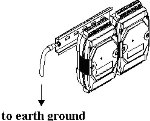
The diagram shows two DRS-125 modules mounted on a DIN rail. A wire is connected to the rail and points downwards with the text "to earth ground".
