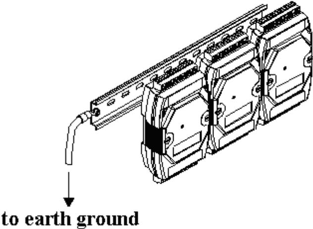
The diagram shows three DRS-240 modules mounted on a DIN rail. A wire is connected to the rail and points downwards with the text "to earth ground".
