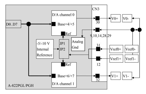
NOTE : The DA output latch registers are designed as "double buffer" structure. <u>The</u> <u>user must send the low byte data first, and then send the high</u> <u>byte data to store the DA 12 bits digital data</u>. If the user only sends the high byte data, then the low byte data will be still the previous value. Also if the user send high byte first then send low byte, the low byte data of DA are still hold in the previous one.
