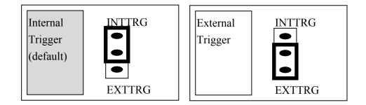
The A-822PGL/PGH supports two trigger type, **internal trigger** and **external trigger**. The external trigger comes from **ExtTrg**, **CN3 pin 17**. There are two types of internal trigger, **software trigger** and **pacer trigger**. The details information is given in section 2.4.8.
