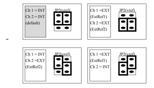
If JP2 select **internal reference**, then JP1 select **-5** V/**-10** V internal reference voltage. If JP2 select **external reference**, then **ExtRef1**, CN3 pin 31, is the external reference voltage for DA channel 1; and **ExtRef2**, CN3 pin 12, is the external reference voltage for DA Channel 2. If user provides AC +/- 10 V external reference voltage, the D/A output voltage may be AC -/+ 10 V
