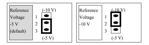
Select (-5 V) : D/A voltage output =  $0 \sim 5$  V (both channel) Select (-10 V) : D/A voltage output =  $0 \sim 10$  V (both channel) JP1 is validate only if JP2 select D/A internal reference voltage
