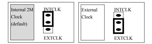
The A-822PGL/PGH has 3 independent 16 bits timer/counter. The cascaded counter1 and counter2 are used as **pacer timer**. The counter0 can be used as a user programmable timer/counter. The user programmable timer/counter can select **2 M internal clock** or **external clock ExtCLK, CN3 pin 37**. The block diagram is given in section 2.6. The clock source must be very **stable.** It is recommended to use internal 2 M clock.
