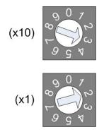
Figure 2-3 Node ID rotary switch
