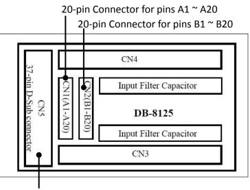
37-pin D-Sub Connector for pins A1  $^{\sim}$  A20 and pins B1  $^{\sim}$  B20
