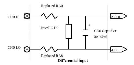
The following is an overview of the resistors/capacitor to be replaced/installed for each channel in differential input mode.
