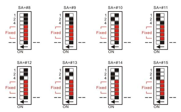
Figure 2.5 Receiver address setting.
