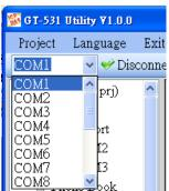
B. Press "Connect" to connect to the GT-531. If the connection is failed, check the COM port settings and wiring.
