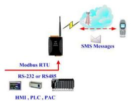
(2) The host sends the Modbus command to transmit the voice alarm from the GT-531.
