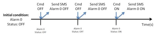
(2) Edge Trigger: When the alarm status change, the SMS will be sent. (It's support Alarm Trigger Time.)
