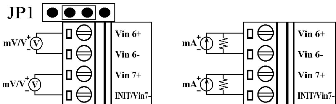
**Note:** When connecting to a current source, an optional external 125-ohm resistor is required.
