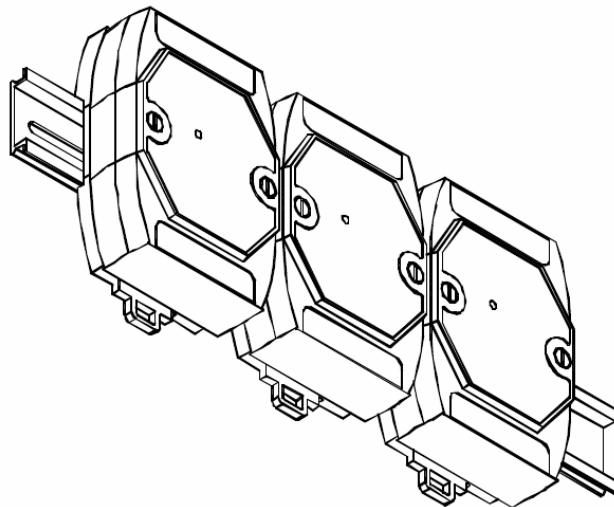
There are three new DIN rail models available. Each are made of stainless steel, which is stronger than those made of aluminum. There is a screw at one end and a ring terminal is included so that it can be easily connected to the earth ground. The three new DIN rail models are as follows.
