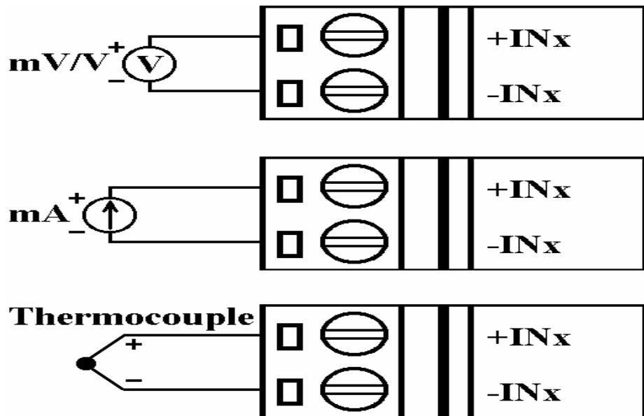
**Note:** When a channel is connected to a current source, the corresponding jumper should be shorted, see Section 1.7.2 for details.
