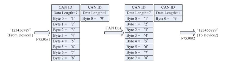
Note: If users use 115200bps for RS-232 port of I-7530A, it is recommended that the configuration of I-7530A CAN baud is closed to the configuration of RS-232 baud, such as 125K bps. When you use pair connection function of I-7530A, the baud under 125K bps is proper.
