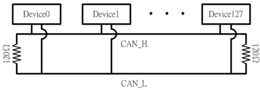
Figure 5: Terminator resistor
