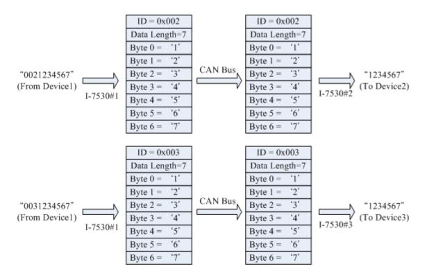
Note: In pair connection mode, all command strings listed in section 4 are useless. When the RS-232/485/422 or CAN buffer of I-7530A is overflow. The ERR Led will be turned on for 300ms, and then I-7530A will be reset by watchdog automatically.
