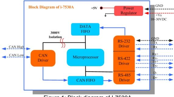
Figure 1: Block diagram of I-7530A
