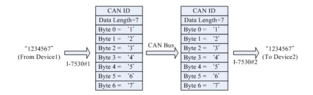
The CAN ID in above figure is determined by the CAN specification selected by users. If users select CAN 2.0A, the CAN ID is 11-bit ID. If CAN 2.0B is used, the CAN ID is 29-bit ID. Here, assume users set the Fixed Tx CAN ID field of I-7530A#1 to be 0x001 ( "0x" is for hexadecimal format) and CAN 2.0A is used, the CAN ID displayed in above figure is 0x001.
