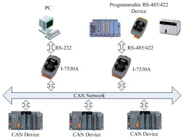
Moreover, we expand the functionalities of I-7530A for some special application. In pair connection mode, I-7530A can be used to connect PC with other RS-232/485/422 devices at the same time. The application architecture may be as follows.
