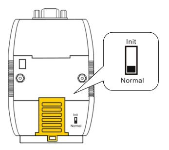
Figure 7: Dip-switch of I-7530A
