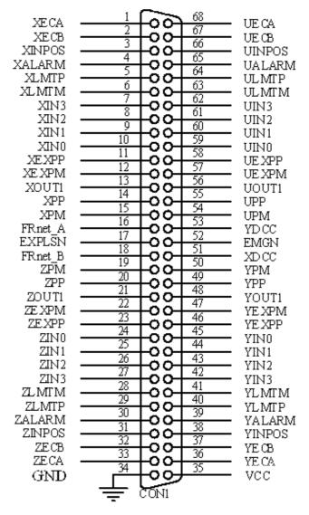
Fig. 2.1 I/O connector pin assignment for the CON1
