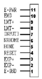
Fig. 7-7 Pin definition for CN1 ~ CN4
