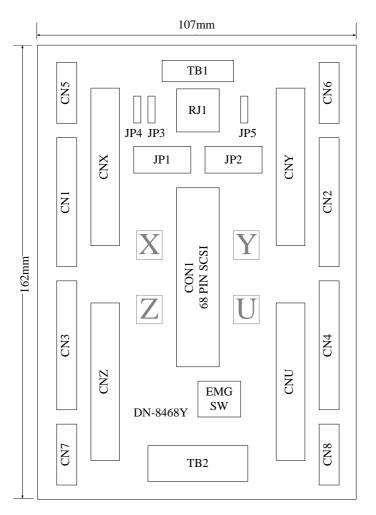
Fig. 3-1 Board layout for the DN-8468Y
