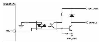
Fig. 2.16 Servo On/Off signal connection diagram
