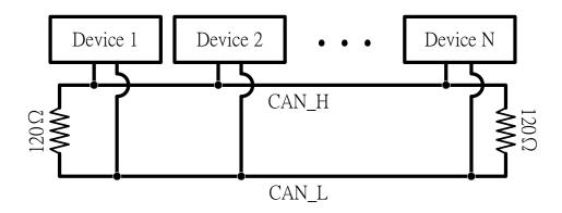
Moreover, to minimize the voltage drop over long distances, the terminal resistance should be higher than the value defined in the ISO 11898-2. The following table can be used as a good reference.
