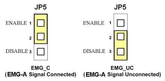
Fig. B3-8 Jumper 5 setting
