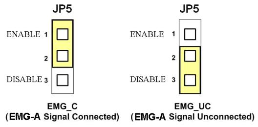
Fig. B1-8 Jumper 5 setting
