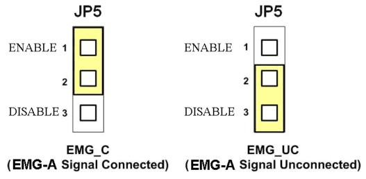
Fig. B4-8 Jumper 5 setting
