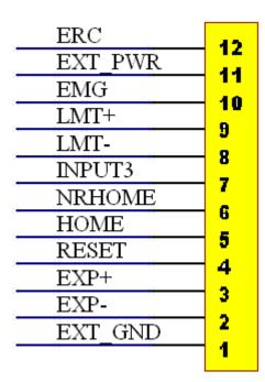
Fig B2-7 Pin definition for CN1~ CN2
