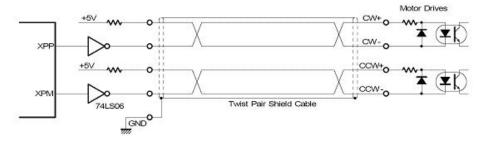
Fig. 2.9 Open-Collector pulse output circuit
