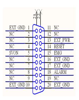
Fig B2-6 Pin definition for CN-XB, CN-YB
