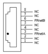
Fig. B3-7 Pin definition for RJ1
