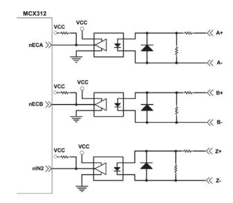
Fig. 2.13 Encoder signal connection
