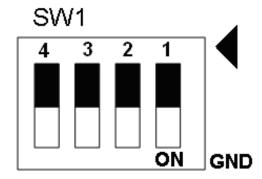
Fig. B1-10 SW1 setting for user controlled signals.
