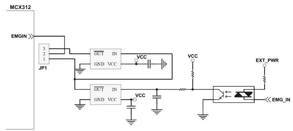
Fig. 2.14 Emergency Stop Signal connection
