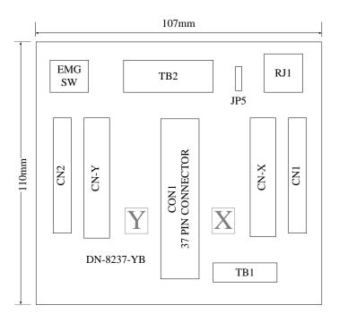
Fig. B4-1 Board layout for the DN-8237-YB
