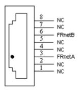
Fig.B4-7Pin definition for RJ1
