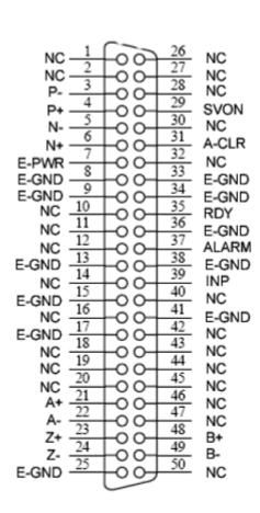
Fig. B3-5 Pin definition for CNX and CNY
