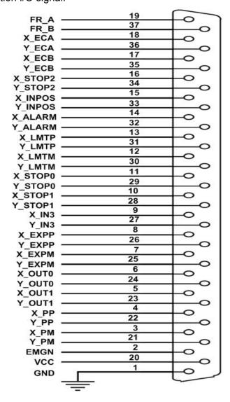
Fig. B4-2 I/O connector pin assignment for the CON1
