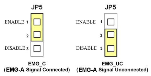
Fig. B2-9 Jumper 5 setting
