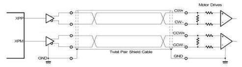
Fig. 2.8 Differential-Type pulse output circuit
