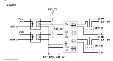
Fig. 2.10 Output pulse example
