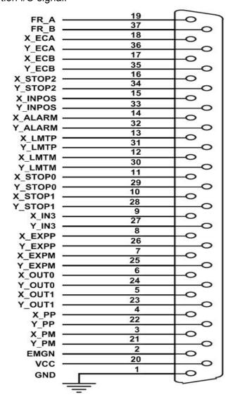
Fig. B2-2 I/O connector pin assignment for the CON1
