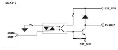
Fig. 2.16 Servo On/Off signal connection diagram
