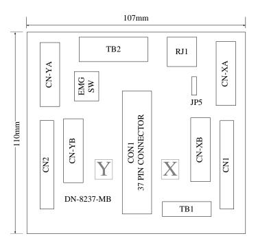
Fig. B2-1 Board layout for the DN-8237-MB
