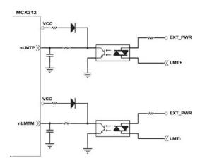
Fig. 2.11 Limit switch signal circuit
