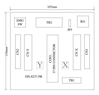
Fig. B3-1 Board layout for the DN-8237-PB
