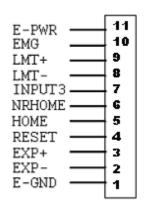
Fig B3-6 Pin definition for CN1 & CN2
