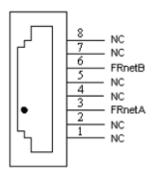
Fig. B1-7 Pin definition for RJ1
