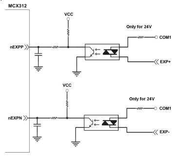
Fig. 2.15 EXP+/- connection diagram
