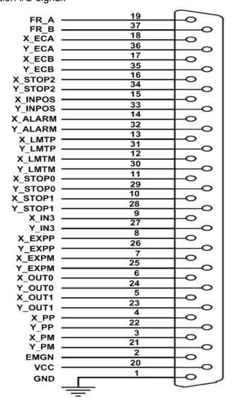
Fig. B3-2 I/O connector pin assignment for the CON1
