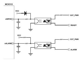
Fig. 2.12 common DI wiring example
