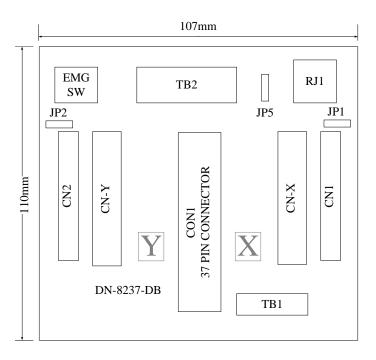
Fig. B1-1 Board layout for the DN-8237-DB
