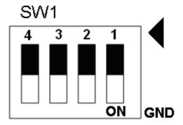
Fig. B2-11 SW1 setting for user controlled signals.
