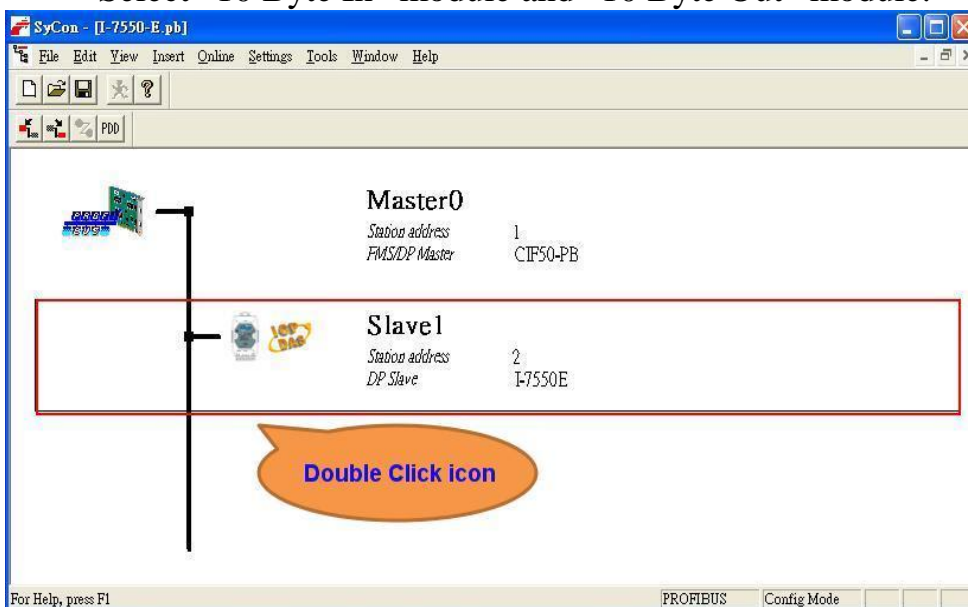
Figure 59 Double click the I-7550E icon to open the “Slave configuration” window
