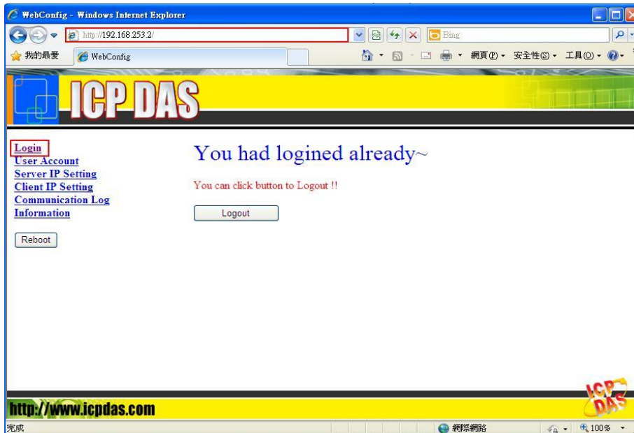
Figure 35 Browser the Web of I-7550E and enter the default password to login.
