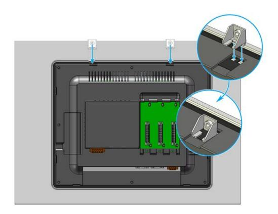
4. Screw the panel mounting clips to the panel.
