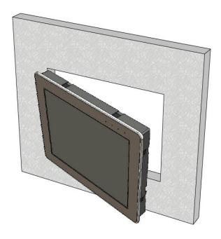
3. Insert the panel mounting clips into the upper and lower ventilation holes.
