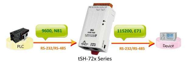
Modbus RTU/ASCII Conversion: This function allows a single Modbus RTU/ASCII master device to communicate with Modbus RTU/ASCII slave devices using different protocols, baud rates and data formats.
