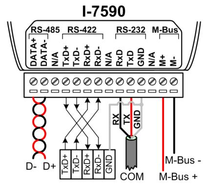
Note: Only one port of the RS-232, RS-422 and RS-485 can work at the same time.
