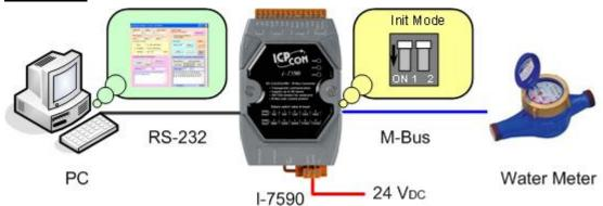
RS-232 Baud rate: 115200 bps (Rotary Switch 9). M-Bus Baud rate: 2400 bps (Rotary Switch 3).
