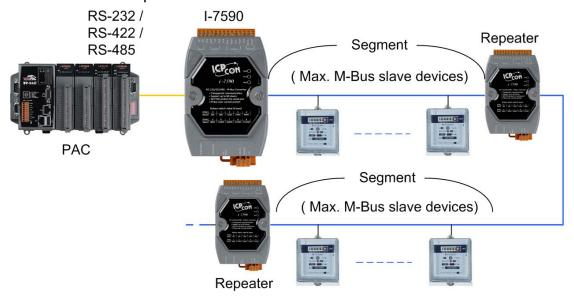
The number of terminals that can be connected to a repeater and the structure of the segments within an extended M-Bus system are determined by the type of cable and the Baud rate.
