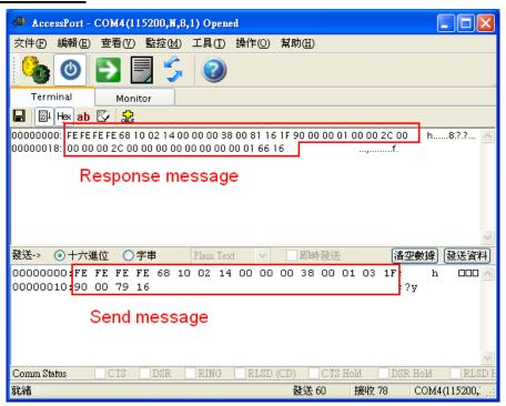
Prepare a software tool which can send and receive binary commands with COM ports, for example SUDT AccessPort as the following website http://www.sudt.com/en/ap/. Send a standard M-Bus command from the PC through RS-232, and I-7590 will pass the command to the M-Bus network and the M-Bus meter will reply the command to the PC.
