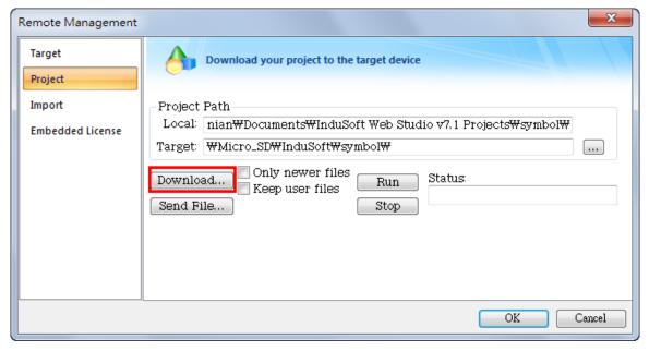
Step 8: The "Files were sent successfully" message will show in the "Status" field when the downloading process finished.
