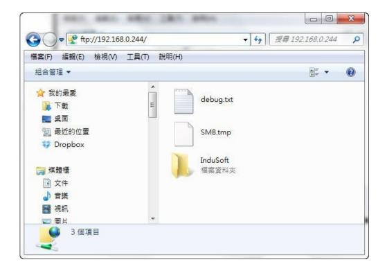
**Step 6**: Copy the InduSoft runtime folder from USB disk to the path, **\Micro\_SD** or **\System\_Disk2** of PAC. Then the updating process is finished.
