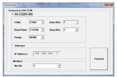
Figure 6: Connection Interface of GW-7238D Utility
