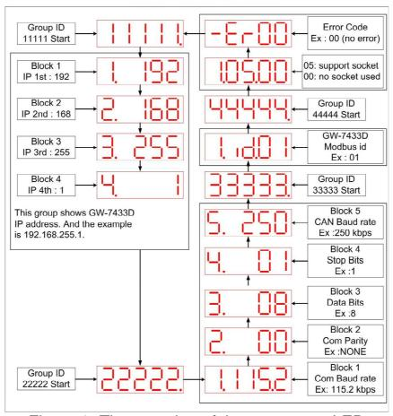
Figure 2: The meaning of the 7-segment LED
