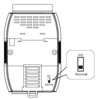
Figure 3: Operation mode Position of Dip-Switch
