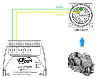
Figure 4: CAN bus Wire Connection
