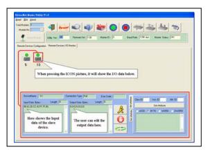
10. Pressing "Refresh output data" button to send the output data to the slave device.
