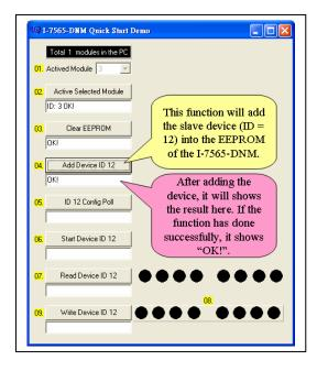
9. In this step, the user can press the "ID 12 Config Poll" button to add the Poll connection information of the slave device (ID = 12) into the EEPROM of the I-7565-DNM.
