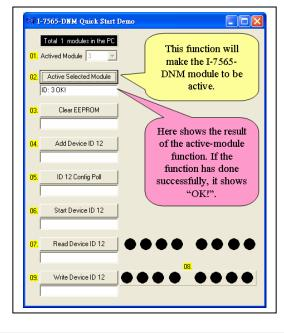
7. In this step, the user can press the "Clear EEPROM" button to clear all setting in the I-7565-DNM. The edit box below will show the result.
