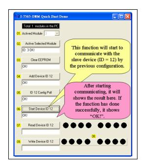
12. In this step, users can press these 8 LED button to edit the output data. And send the data to the output channel of the slave device (ID = 12) by pressing "Write Device ID 12" button to send the output data to the output channel of the slave device (ID = 12). At the same time, the D/O LED on I-8077 will show the same value.
