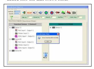
7. Pressing "Start all Device" button to communicate with all slave devices. We can ignore the warning message in this example.
