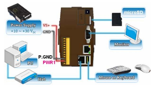
□ The diagram below shows the connections of LP-8441/ LP-8841.
