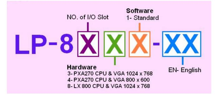
The LP-8x4x model type is shown in the above figure. The Second number shows the slot numbers coming with the main controller unit. Currently, we provide three types of  $1 \cdot 4$  and 8 slots. The last number demonstrates the application platform. 1 stands as the Master controller and it means that the user needs to design the application program.
