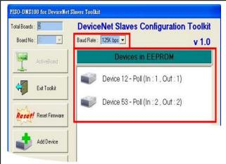
3. Pressing "Clear All Config" to clear unknown information. This button would also reset the baud rate to the default value (125K). It pops up a dialog to make sure that you want to clear them. After clearing successfully, the users should change the baud rate to the original setting.
