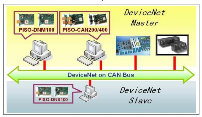
The users should prepare at least one DeviceNet master for demonstrating the I/O data exchanging. The users can use the PLC with DeviceNet master module to start this demo. There are some DeviceNet master products provided by ICPDAS, such as PISO-DNM100U, PISO-CAN 200/400...etc. Please visit the following web site for more information.
