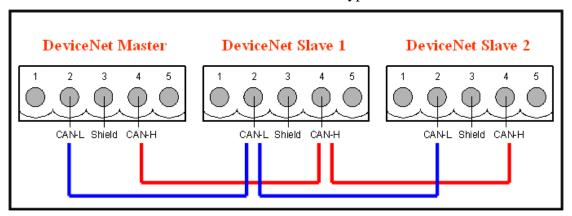
The following wire connection is **wrong** which is shown as follows.
