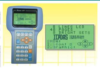
The iVIEW-100 series can be also used as a HMI device for our I-7188,  $\mu$ PAC-7186 and I-8000 series embedded controller. Since the basic hardware design of iVIEW-100 is similar to that of I-7188 series, all our available software can be used in iVIEW-100. User can design iVIEW-100 application with C Language. We will provide iVIEW-100E with a 10/100 mega Ethernet port for internet.
