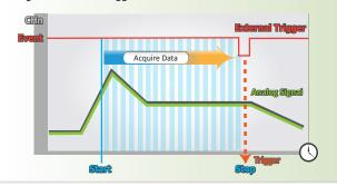
Delay-trigger Mode: In delay-trigger mode, signal capture begins once the programmed delay period from the trigger has elapsed.
