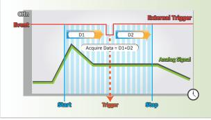
Pre-trigger Mode: In pre-trigger mode, the signals are digitized before a trigger condition occurs.
