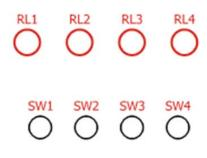
SW1 ~ SW4 are test push buttons that control Relay 1 ~ Relay 4 ON / OFF.
